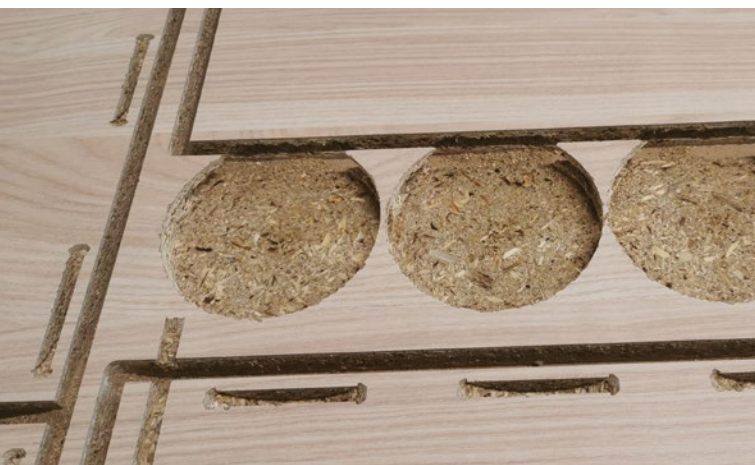
Milling for the Lamello TENSO connector on both the surface and the edge.
