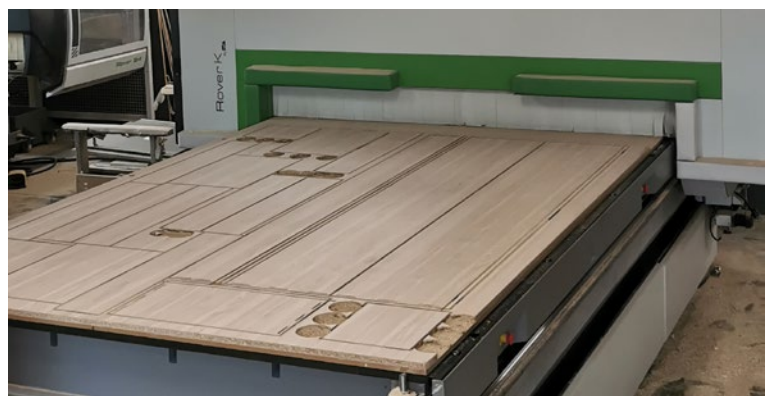
The Biesse Rover K FT nesting machine is very space-efficient and allows for access from all sides.
